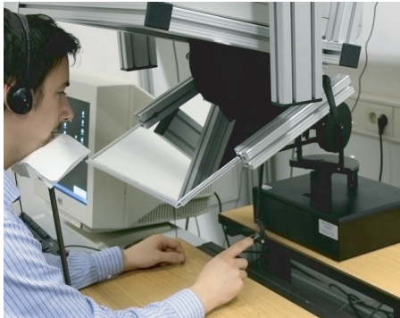
Figure 1: Experimental set-up. Visual stimuli were presented on a CRT monitor and mirrored to appear aligned with haptic stimuli. Haptic stimuli presentation was controlled by a PHANToM device, and the visual stimuli were generated by OpenGL with the GLUT toolkit. The participant's head position was fixed by the aid of a chin rest, ensuring a stable viewing distance of 57 cm to the mirror display surface.
