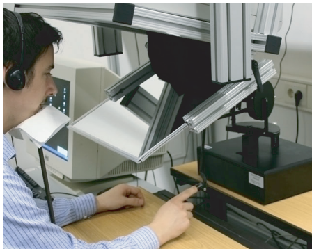
Figure 1: Experimental set-up. Visual stimuli were presented on a CRT monitor and mirrored to appear aligned with haptic stimuli. Haptic stimuli presentation was controlled by a PHANToM device, and the visual stimuli were generated by OpenGL with the GLUT toolkit. The participant's head position was fixed by the aid of a chin rest, ensuring a stable viewing distance of 57 cm to the mirror display surface.
